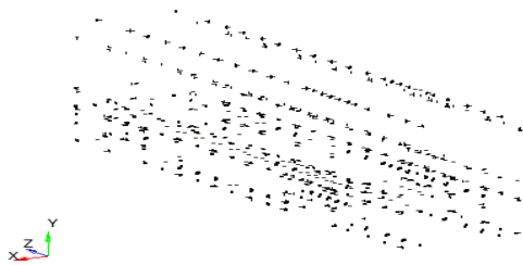
Figure 4: Bus rigid welding RBE2
